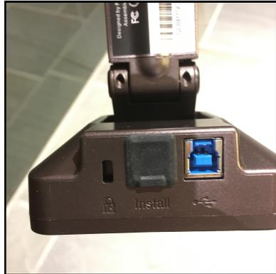
2. Plug the orange cable into *Install* port (you may need to first remove cable from SB port to right of *Install* port).
