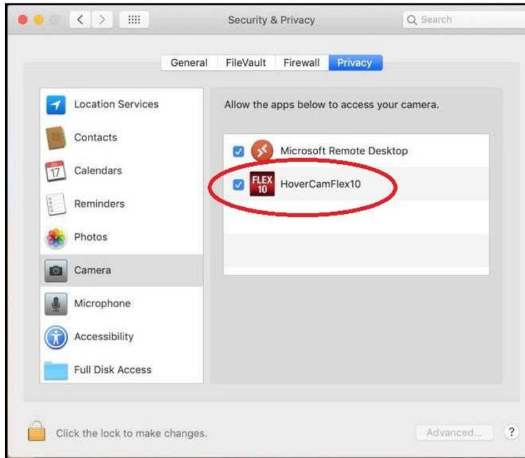
d. Click the lock icon in the bottom left corner to unlock access; it should change to show an unlocked padlock icon. Check the box next to HoverCamFlex10 to allow the Hovercam to access the laptop's camera for displaying images.
