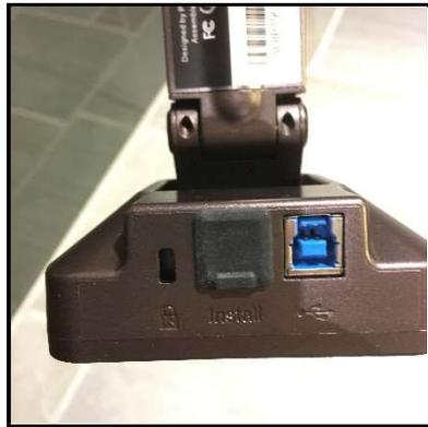
2. Plug the orange cable into *Install* port (you may need to first remove cable from USB port to right of *Install* port).
