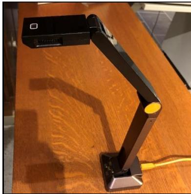
2. Turn on Hovercam lights if desired, by sliding switch on side of camera neck.
